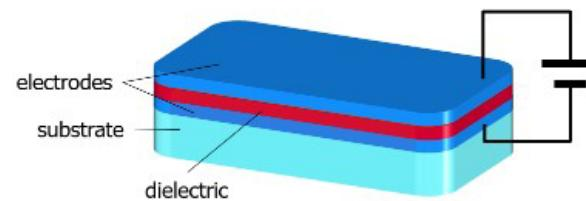
Resistive switching (RS) occurs when a dielectric material undergoes a rapid and non-volatile change from high to low resistance or vice versa.
