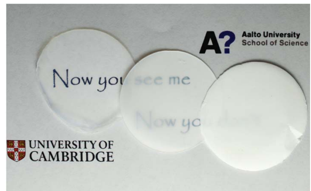
Figure 2 – White cellulose films made using the structural colour technology
