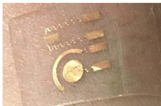
Fig. 3: Conformable and biocompatible skin sensor prototype
